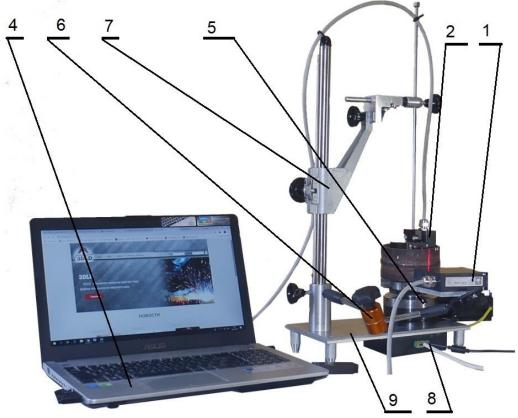
The LST scanner is designed for non-contact measurement and digitization of the front and root surfaces of the weld of butt of test pipes, for subsequent assessment using 3DLD technology of the practical skills of fusion welding welders.
