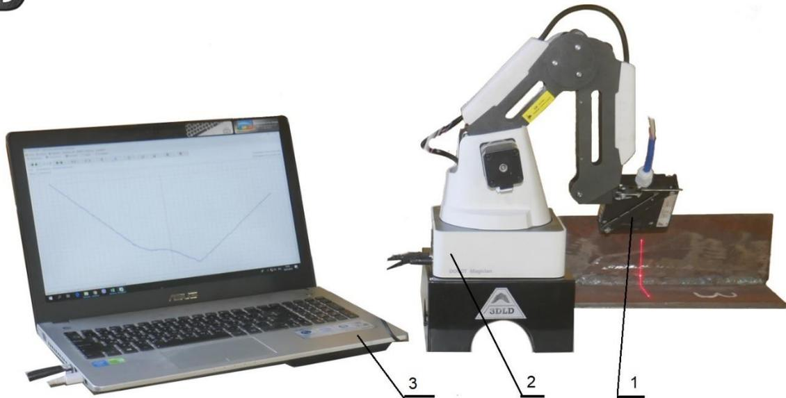
The LSR scanner is designed for non-contact measurement and digitization of the weld surface of butt and corner test plates, for subsequent assessment using 3DLD technology of the practical skills of welders in fusion welding.
